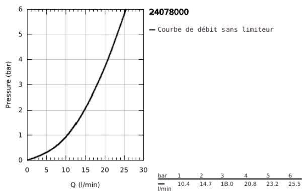
24 078 000 GROHTHERM MITIGEUR THERMOSTATIQUE 1 SORTIE AVEC VANNE D'ARRÊT
