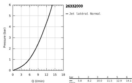
26 332 000 **SENA TRIGGER SPRAY 35 ENSEMBLE AVEC ROBINET D'ARRÊT 1 JET**
